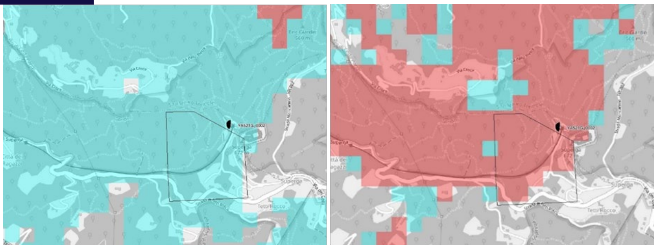
Figure 9. Simulation of the coverage level by installing the new BTS in Turin.
