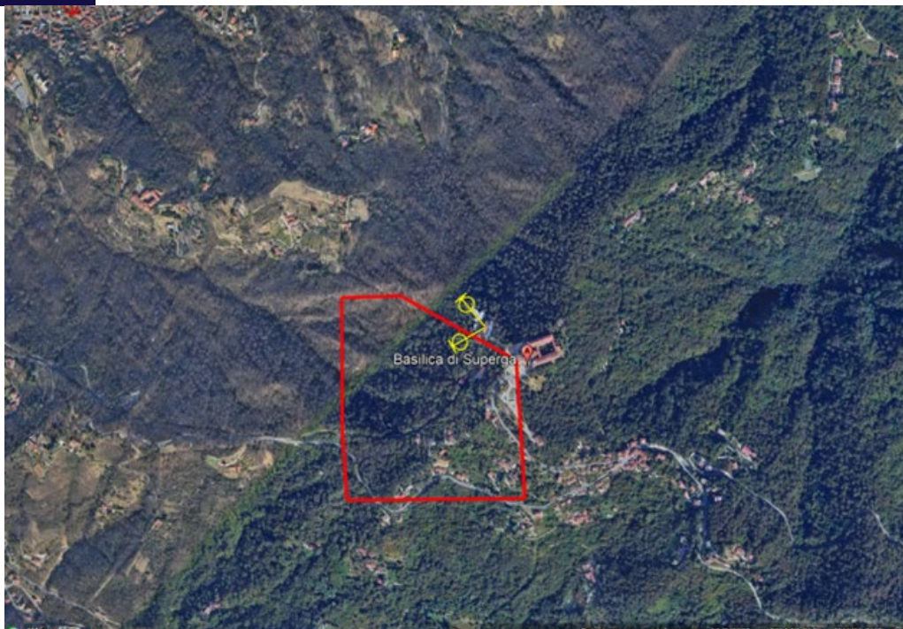
Figure 11. The estimated position of the BTS, the azimuth of 2 sectors, and the flying test area (red polygon).
